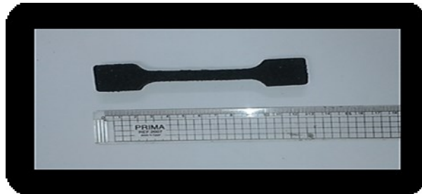
Figure 1 the tensile testing specimen of the polyurethane- based composite solid propellant
