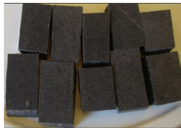
Figure 2 density specimen of the polyurethane- based composite solid propellant
