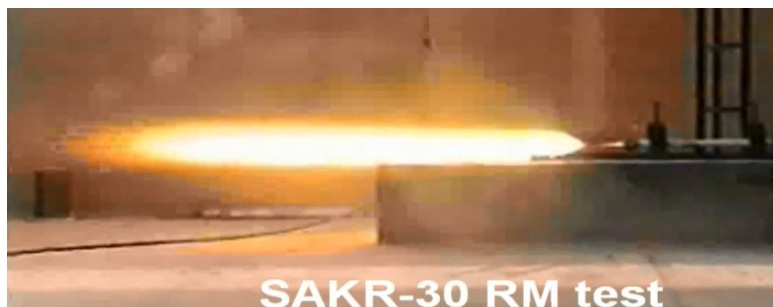
Fig. (2) Static firing test and a typical configuration of real 122mm RM with composite SP grain
