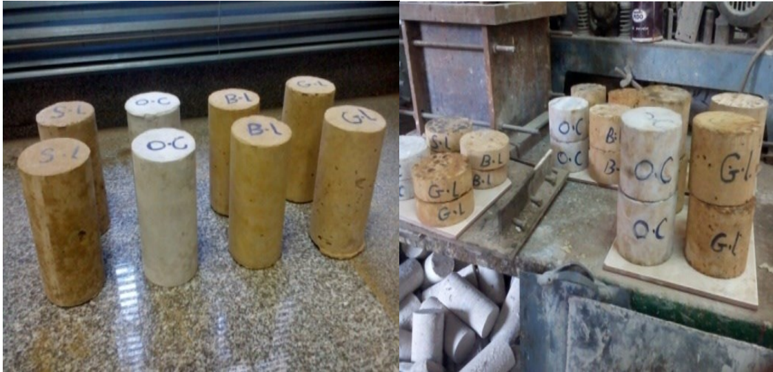
Figure 5: The cylindrical samples used for gamma rays attenuation measurements.
