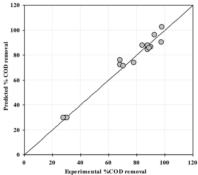
Fig.2. Predicted vs. experimental data for COD removal (%) ( $R^2 = 0.97$ )
