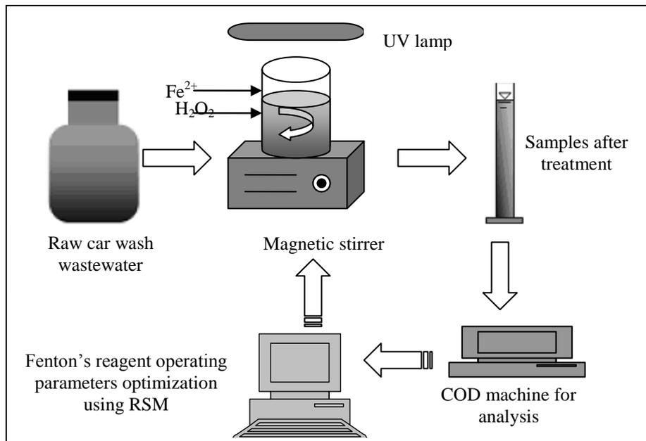
Fig. 1. Schematic diagram of lab-scale photo-Fenton test
