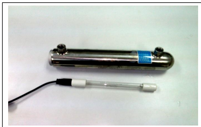
Fig.1. The photochemical cell used in the photocatalytic process
