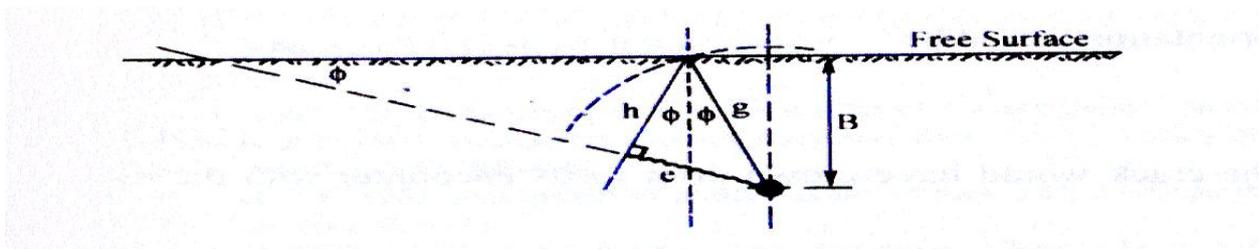
**Figure (2): Favorable reflection geometry for extending cracks toward the free surface**
