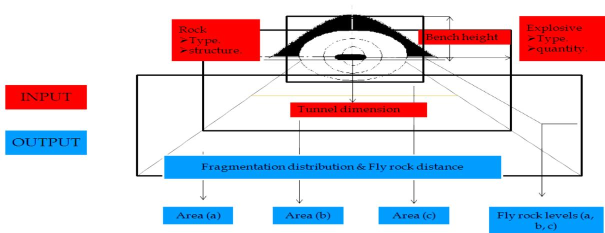
Fig. (3) Input and Output Data for Central Blasting
