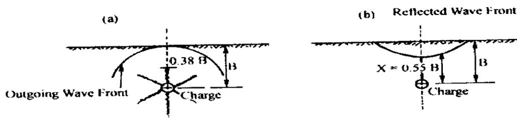
**Figure (1): Diagrammatic representation of the interaction of spherical wave with the radial cracks system.**
