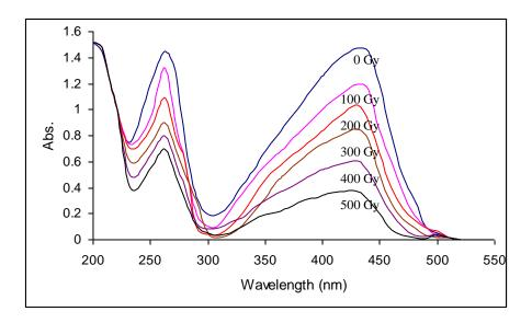
Figure 2: UV–Vis Tartarzine absorbance spectra for different doses (0 to 500 Gy), concentration =  $5 \times 10^{-4}$  M and pH = 9.
