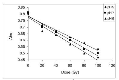
Figure 6: shows that Tartarzine of concentration  $10^{-4}$  M is more bleached after 24 hours of primary irradiation especially at pH 9
