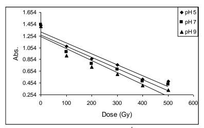
Figure 7: shows that Tartarzine of concentration  $5 \times 10^{-4}$  M is more bleached after 24 hours of primary irradiation especially at pH 9
