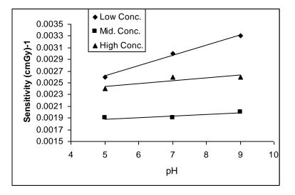
Figure 10: Dependence of sensitivity on the pH value of Tartarzine solution.
