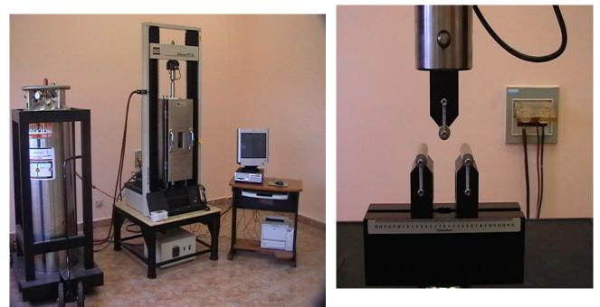
Figure 1: RT30 Material Testing System used for compression and flexural tests
