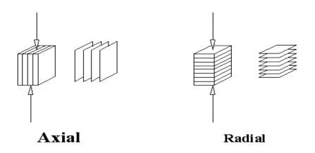
Figure 3: Axial and radial compression specimens for composite material
