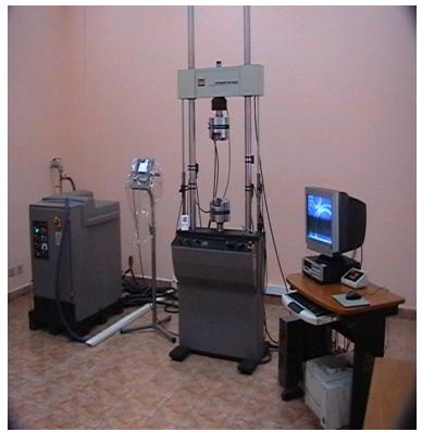
Figure 2: MTS810 Material Testing System used for tensile test
