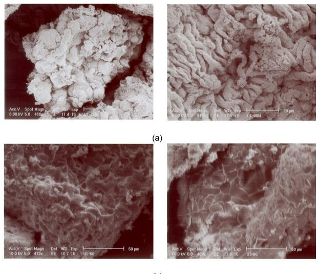
(b) Fig. 2. The SEM of zinc oxide prepared by sol-gel technique calcined at (a) 500°C and (b) 700°C
