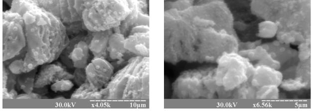
Fig. 3. The SEM of zinc oxide prepared by Pechini calcined at 700°C
