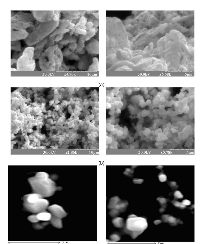
Fig. 4. The SEM of zinc oxide prepared by Pechini calcined at (a) 900°C and (b) 900°C for 6 hrs
