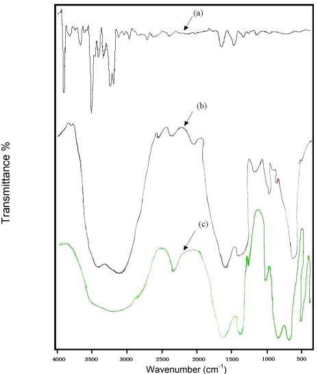
Fig.5. The IR spectrum of the samples prepared at room temperature and dried at 100°C (a) by Pechini (b) via sol-gel and (c) pure zinc acetate dihydrate
