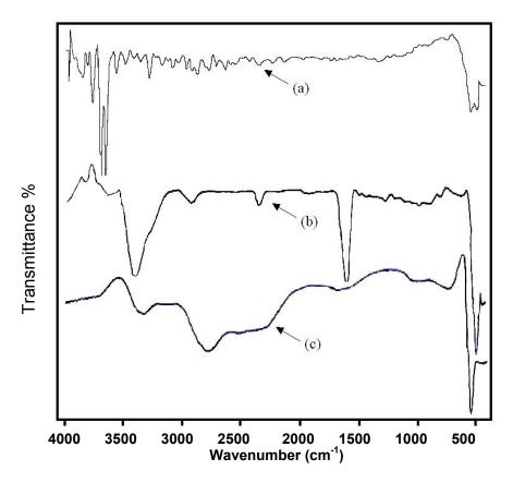
Fig.6. The IR spectrum of the samples calcined at 900°C (a) by Pechini (b) by sol-gel, (c) pure zinc oxide
