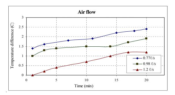
Fig.3. Effect of volumetric air flowrate between two idetical samples treated with emulsion paint and Al spray on temperature difference of a hot plate and background with time.
