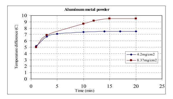
Fig.1. Effect of textile barrier treated with emulsion paint and different weights of Aluminum powder on temperature difference of a hot plate and background with time.
