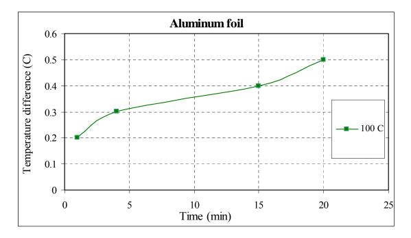
Fig.4. Effect of a singe AI foil sheet on temperature difference of a hot plate and background with time.
