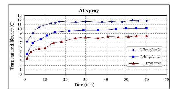
Fig.2.Effect of textile barrier treated with emulsion paint and different concentrations of AI spray on temperature difference of a hot plate and background with time.
