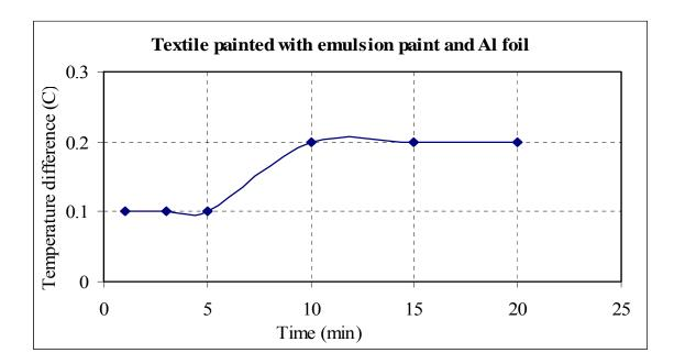
Fig.5. Effect of alminum foil sheet supported on a textile sample treated with plastic paint on temperature difference of a hot plate and background with time.
