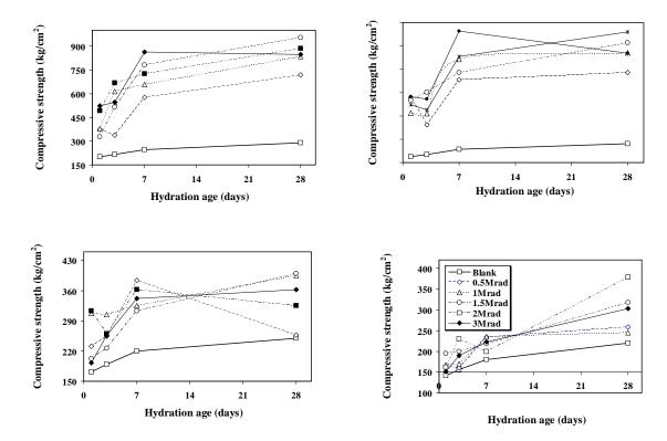
Fig.(4): Compressive strength (kg/cm<sup>2</sup>) of the hardened OPC mortar pastes impregnated with polyurethane (C.O. + MDI) – MMA copolymer at different doses of  $\gamma$ -rays as a function of the hydration age, (W/C ratios 0.25, 0.30, 0.40 and 0.50).
