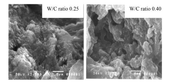
Fig. (3): SEM micrographs of the hardened cement mortar pastes made of OPC impregnated with polyurethane (MDI + C.O.), (W/C ratio 0.25 & 0.40), hydration time 28 days.
