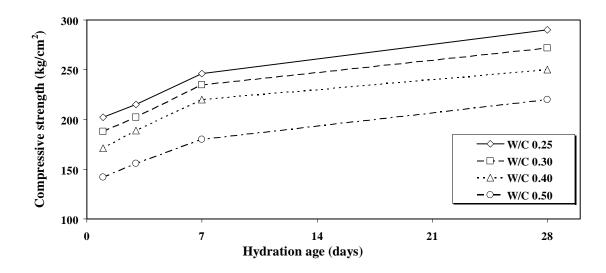
Fig. (1): Compressive strength (kg/cm2) of the hardened neat OPC mortar pastes made by using different W/C ratios (blank) versus age of hydration.
