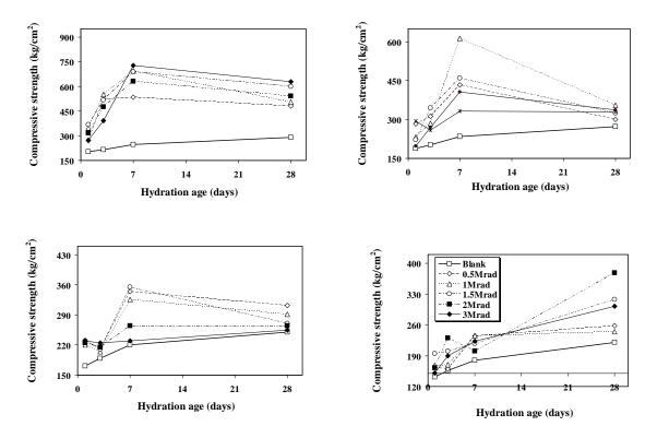
Fig.(2): Compressive strength (kg/cm2) of the hardened OPC mortar pastes impregnated with polyurethane (C.O. + MDI) at different doses of  $\gamma$ - radiation as a function of the hydration age, (W/C ratios 0.25, 0.30, 0.40 and 0.50).
