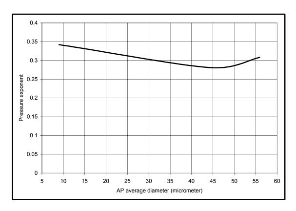
Fig.9. Effect of AP particle size on the pressure exponent.
