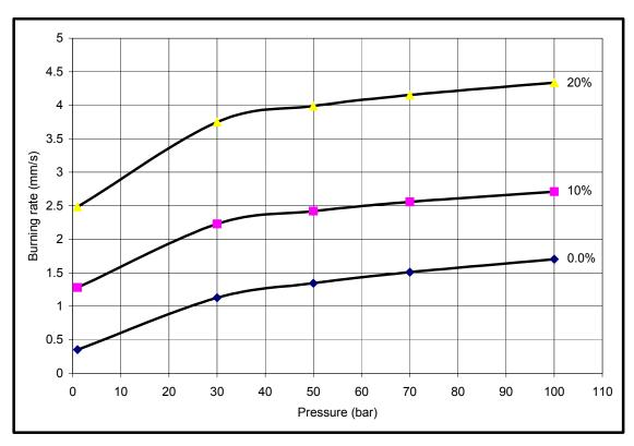
Fig.10. Burning rate versus pressure at different Al contents.
